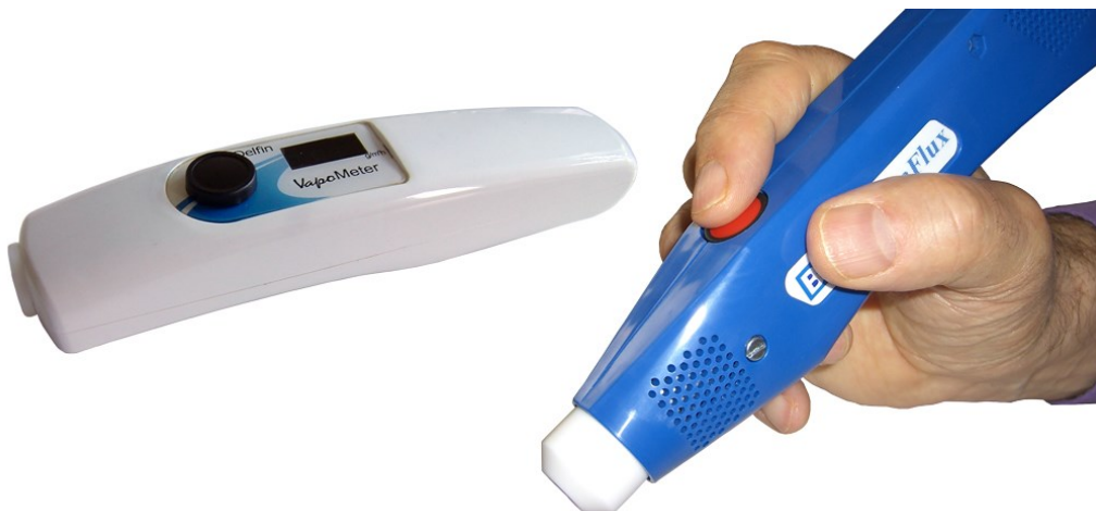
Figure 1: The two closed-chamber instruments used in the study. Left: Unventilated-chamber VapoMeter. Right: Condenser-chamber AquaFlux.
