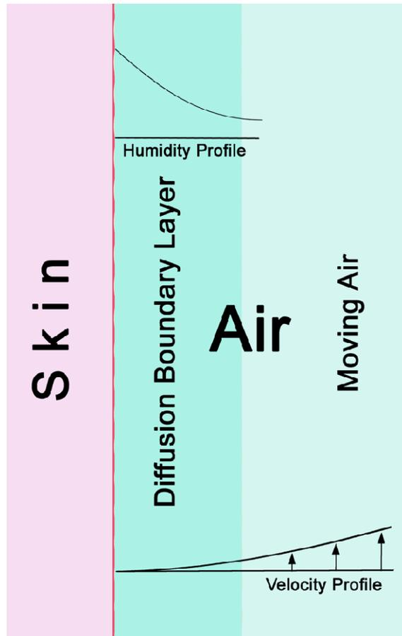
Water evaporates from the SC surface into the adjacent air. The air immediately next to the SC surface forms a **diffusion boundary layer** of still air [4]. The moving air next to the diffusion boundary layer acts as a **vapour sink** of constant humidity and temperature.
