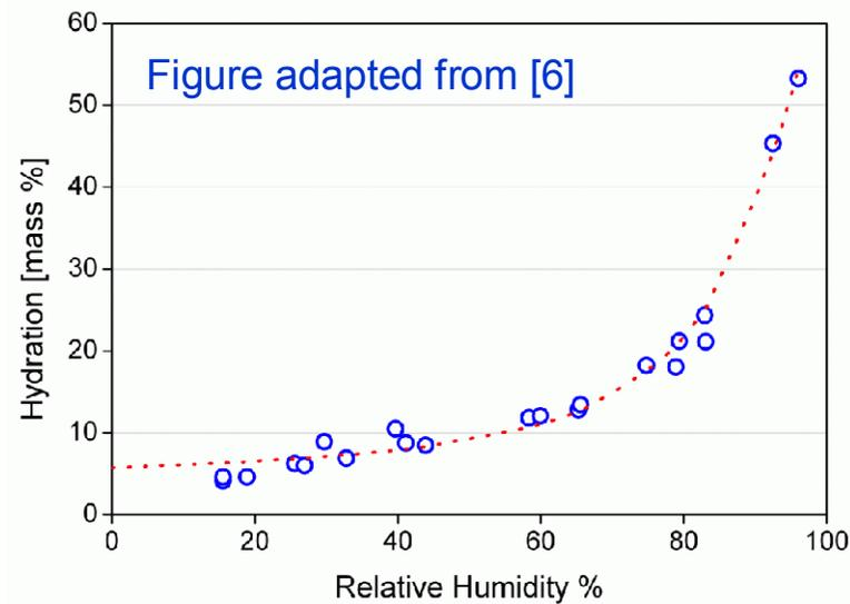
Adsorption & desorption processes at the SC surface maintain a balance between the **hydration** of the SC and the **humidity** of the adjacent air.
