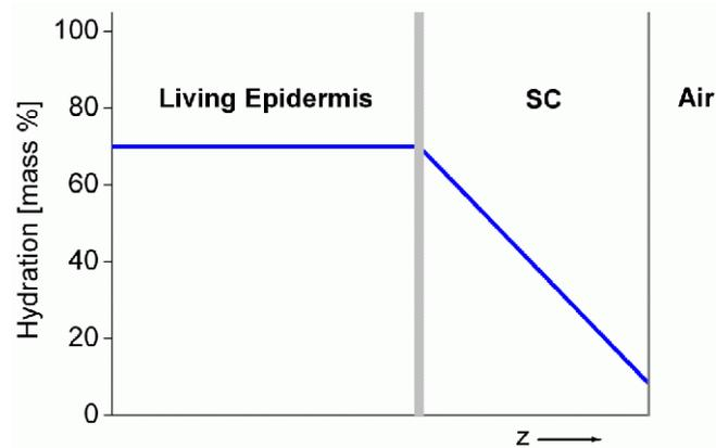
Hydration depth profile of the proposed new model, assuming a uniform SC.
