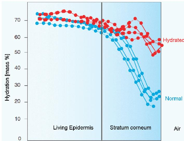
Hydration depth profiles measured using confocal Raman spectroscopy.
