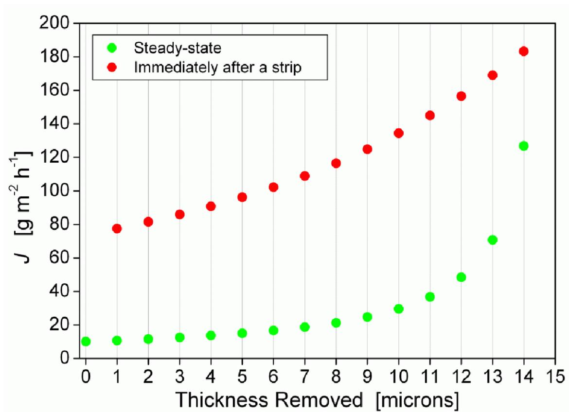
The transient vapour flux is calculated immediately after strips of 1  $\mu\text{m}$  thickness.
