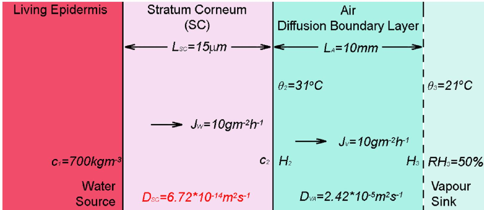
The parameters in **black** were used in this example calculation. They are sufficient to determine the diffusion coefficient of the SC,  $D_{SC}$ , for an assumed TEWL of  $10 \text{ g m}^{-2} \text{ h}^{-1}$  for intact SC.
