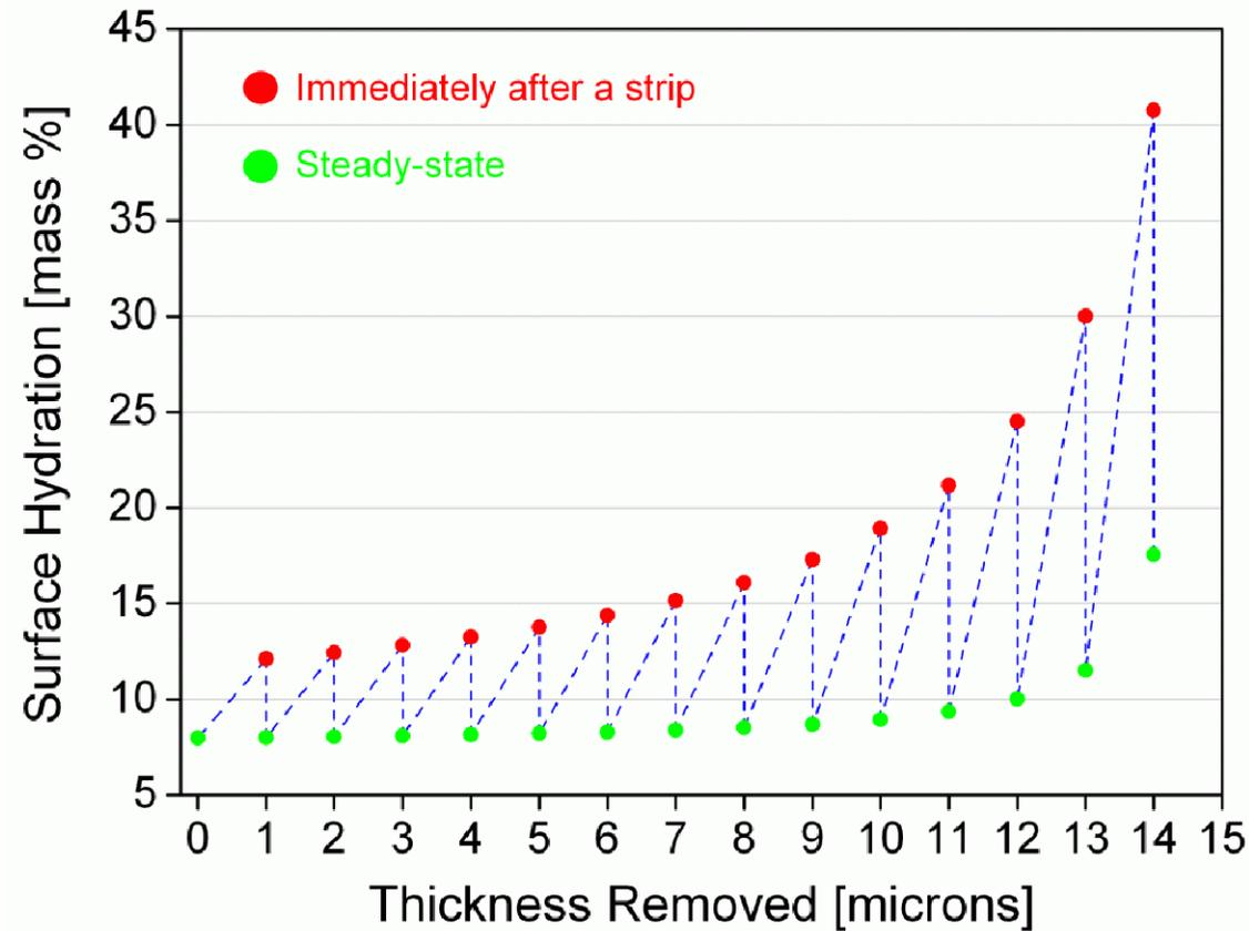
This figure shows calculated transient & steady-state SC surface hydration with 0, 1, 2, ... microns of SC removed by stripping. The excess hydration immediately after a strip is subsequently lost by evaporation from the SC surface (=Skin Surface Water Loss, SSWL).
