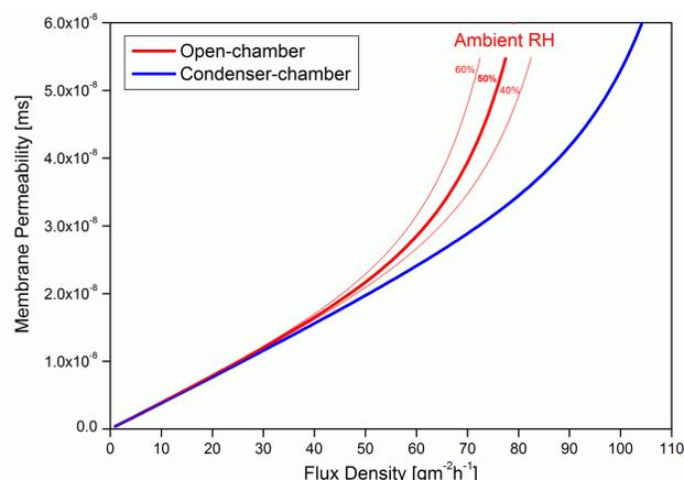
**Figure 1: Model calculations of the relationship between flux density and membrane permeability for typical open-chamber and condenser-chamber instruments.**
