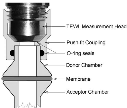
**Figure 2: TEWL Measurement Head coupled to a glass Franz cell for membrane integrity testing.**
