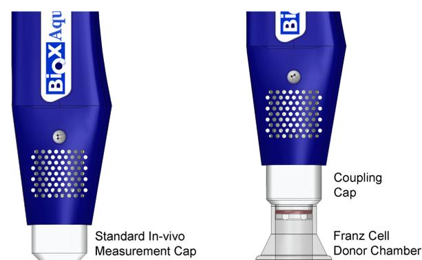
**Figure 3: AquaFlux instrument equipped with a standard in-vivo measurement cap (left) and coupled to a 15mm Franz cell donor chamber (right). The cap-factor calibration method compares same-site readings on in-vivo skin.**
