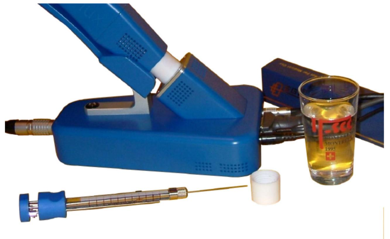
Figure 1: Droplet method for testing solvent effects on TEWL measurement.
