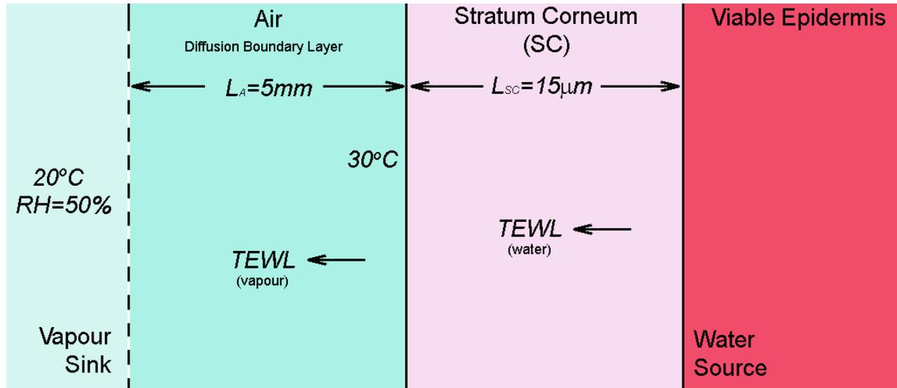
This diagram represents the model, together with some of the values used in the calculations that follow. These were performed using the Excel 2003 spreadsheet and its VBA (Visual Basic for Applications) feature. Properties were calculated layer by layer, dividing the SC into 1000 layers. A typical diffusion coefficient was found to be 0.15% smaller with 500 layers and 0.07% larger with 2000 layers.
