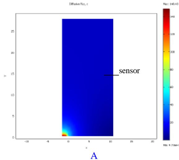
**FIGURE 3.** Finite Element simulation of water vapour flux density map within a TEWL measurement chamber. A: droplet at the edge. B: droplet at the centre. C: with a longer chamber.
