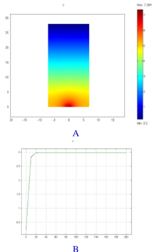
**FIGURE 2.** Finite Element simulation of water vapour density map within a TEWL measurement chamber. A: vapour density at 200sec. B: vapour density vs time (sec) at the sensor position. Water vapour diffusion coefficient of air used is  $2.54 \times 10^{-5} \text{ m}^2/\text{s}$ .
