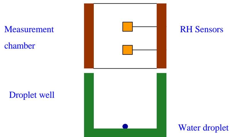
**FIGURE 1.** Schematic diagram of the droplet method used to calibrate a TEWL instrument.
