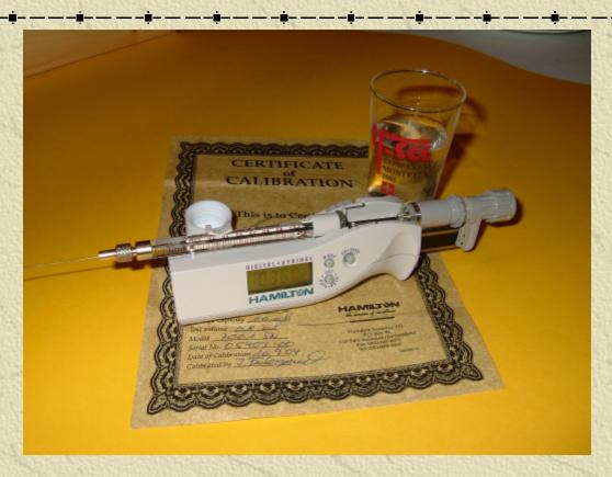
Traceability is provided via a calibrated micro-syringe such as the one shown above.
