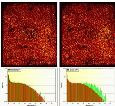
**Figure 3:** These two images are the same, but with the 2.6mm diameter green Region of Interest (RoI) circle displaced by a horizontal distance of 3.8mm.
