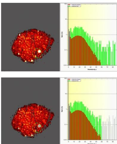
**Figure 5:** The yellow/white spots are surface water from imperceptible perspiration. The 2mm diameter green *RoI* encloses an area where surface water predominates. Within this *RoI*, the mean permittivity is considerably higher ( $\epsilon \sim 27.8$ , CV  $\sim 78\%$ ) than for the whole area of contact.
