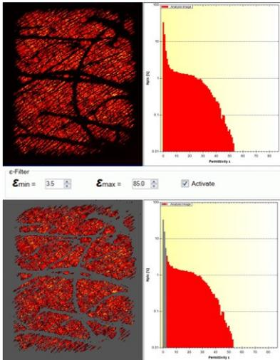
**Figure 4:** Hairy male ventral forearm, where the bad contact shows up as black, ie low  $\epsilon$  of hair and air. The histogram (NB: Log scale) indicates bad contact by the prominent peak at low  $\epsilon$ .
