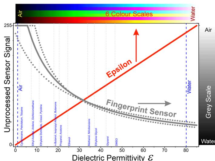
**Figure 1: Native capacitance response (grey) and calibrated permittivity response (red) of a typical fingerprint sensor.**
