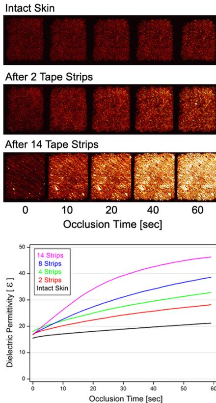
**Figure 6:** Shown here are example images from the recorded bursts. Note that significant barrier damage becomes visible after just 2 strips, as indicated by the increased rate of surface water accumulation compared with intact skin. Also, the barrier damage after 14 strips is highly heterogeneous, with the bright yellow areas indicating greater than average damage.
